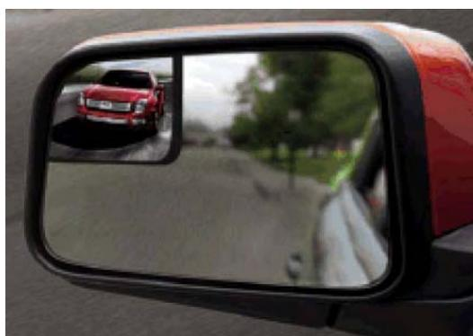
*Figure 12: FMVSS 111 compliant planar main viewing mirror with a voluntarily fitted blind-spot viewing auxiliary wide-angle mirror (Lynam, 2009)*
